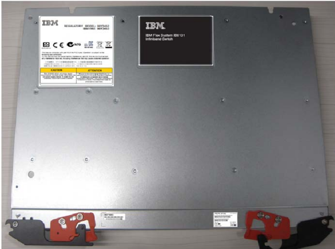
Figure 2: Switch label location
