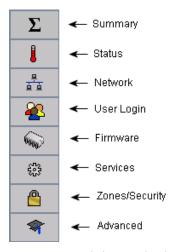
Figure 14. Switch data window buttons
