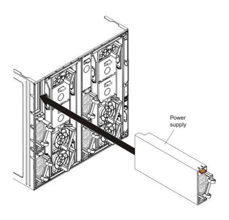
Figure 1. 2100 W / 2500 W Power® supply
